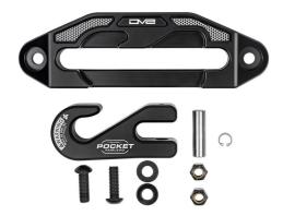
STEP 1 | Pull the winch line through the fairlead and secure the fairlead to the bumper using the provided 1/2" hardware with a 5/16" allen bit and 3/4" wrench.
