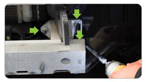
**STEP 15** Using your pefered cutting tool, cut the grille support bracket as shown.
