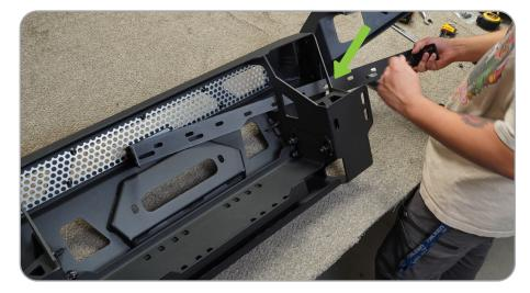
**STEP 23** | Place the light bar bracket so that the mounting tabs are inside the bumper mounting tabs.
