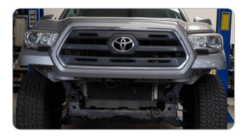
STEP 27 | Place your bumper onto the vehicles crash bar studs. Using the factory nuts removed on step 14 and a 14mm socket or wrench, loosely secure the bumper.
