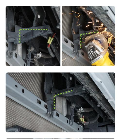
STEP 16 Unbolt the power steering cooler from the frame. Use the provided relocation brackets with the provided M8 hardware to move the cooler closer to the A/C Condenser.
