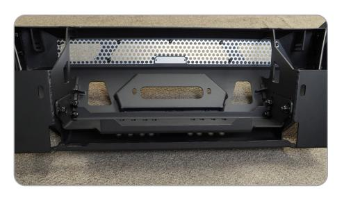
STEP 22 | If you plan on running a light bar, install the light bar bracket at this time.
