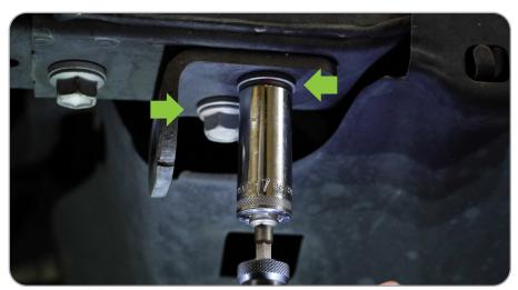
**STEP 18** Using the 17mm socket, remove the remaining bolt on the underside of the front frame crossmember to remove the frame extension. Repeat on opposite side.
