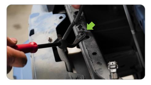
**STEP 8** I In each fender, remove the first two bolts closest to the front of the vehicle using an 10mm. There are two clips securing the front section of the fender to the bumper. To remove these clips, reach inside the wheel well and squeeze the pushdown tabs and push clips out.
