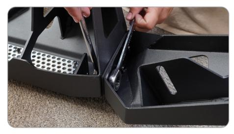
STEP 21 | If running a winch, install the winch onto the winch plate prior to installing the winch plate onto the bumper. Use the hardware provided with the winch to mount the winch.
