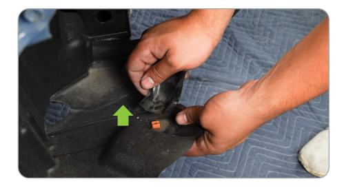
STEP 11 | Disconnect the wheel well orange clips crash bar support
