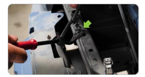
STEP 8 In each fender, remove the first two bolts closest to the front of the vehicle using an 10mm. There are two clips securing the front section of the fender to the bumper. To remove these clips, reach inside the wheel well and squeeze the pushdown tabs and push clips out.
