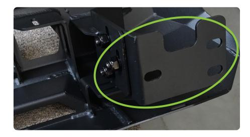
STEP 25 | If you are planning to run pod lights install them at this time using the hardware provided with the lights.
