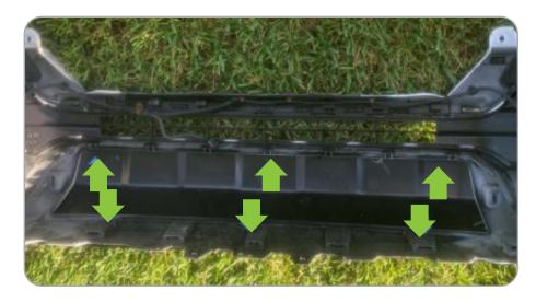
STEP 18 | With the center portion removed, re-install the lower bumper portion and secure using the factory hardware and trim clips.
