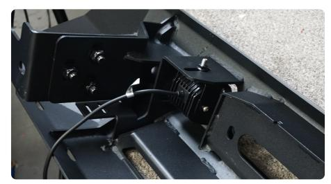
STEP 26 | If you are running a winch install the fairlead at this time using the hardware provided with the fairlead.
