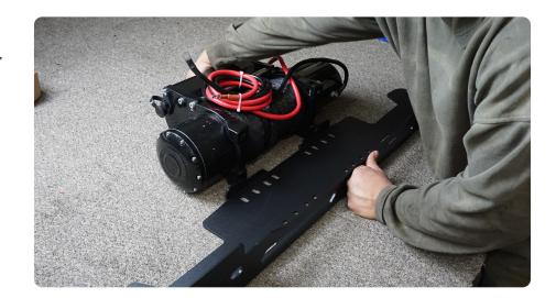
STEP 28 | Lift the winch plate/winch up to the vehicle and loosely secure using the factory hardware.
