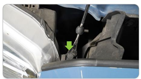
STEP 3 | Use the push pin removal tool to unplug the air sensor harness on the backside of the grille.
