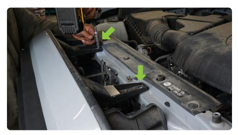
$\begin{array}{c|c} \text{STEP 32} & \text{Re-install the factory push} \\ \text{clips securing the grille to the vehicle.} \end{array}$
