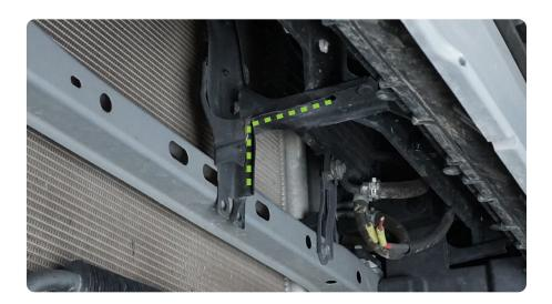
STEP 23 | Unbolt the power steering cooler from the frame. Use the provided relocation brackets with the provided M8 hardware to move the cooler closer to the A/C Condenser.
