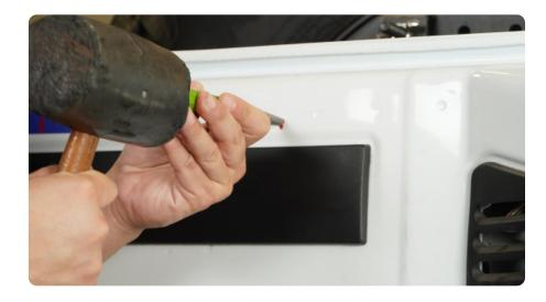
STEP 6 | Drill the mounting holes out using a 11/32 drill bit.
