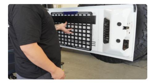
STEP 4 | Mark the mounting holes within the large slotted cutouts at the edges of the molle panel.
