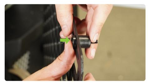
STEP 9 | Loosely secure the molle panel to the vehicle using two of the provide M6 bolts, washers and spacers.
