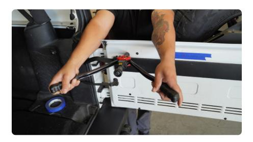
STEP 8 | Thread the provided M6 counter sunk bolt through the counter sunk washer, and through the molle panel.
