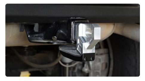
STEP 3 | DV8 offers replaceable skid pads (Aluminum or Delrin) Part# UNHS-APAD/ UNHS-DPAD.
