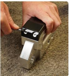
STEP 2 | Using your chosen 5/8" hitch pin, install the hitch skid into your tow hitch receiver.
