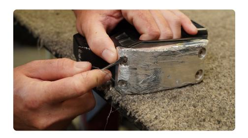
STEP 4 Using a #4 allen tool, remove the (4) M6 counter sunk allen head bolts and remove the damage skid pad.
