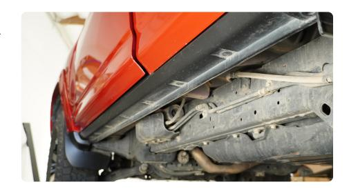
STEP 2 | The DV8 OE plus steps will mount to the vehicle rocker panel, using the (6) threaded factory accessories holes.
