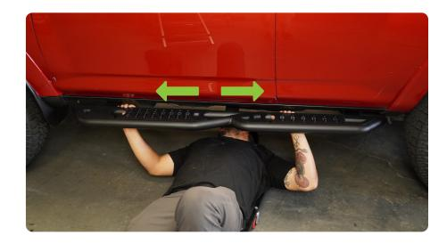
STEP 4 | Align the steps mounting brackets with the factory accessories holes.
