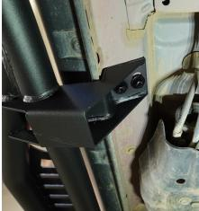
STEP 5 | Adjust the steps forward and back to your preference. Using a 13mm socket secure the step in place.
