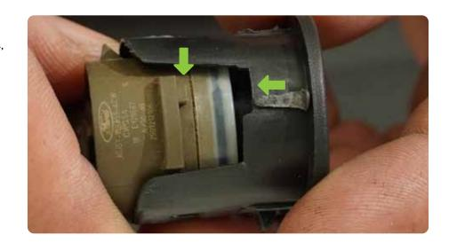
STEP 3 | This shows an example of the sensor fully seated in the bezel.
