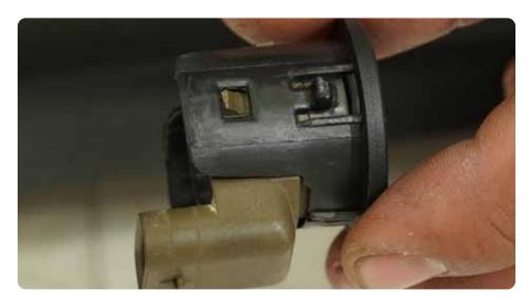
STEP 4 | With the sensor removed from the bezel, place the bezel into the bumper from the front side (noting the correct orientation).
