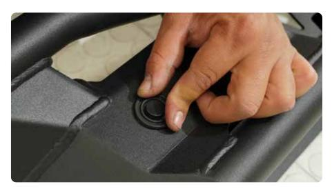
STEP 6 Once all are set into place, reconnect sensor and check to ensure orientation is correct and sensor is evenly spaced in the bezel.
