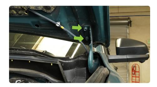
STEP 2 | Using a 12mm socket, loosen (2) of the hood hinge bolts about 40% loose.
