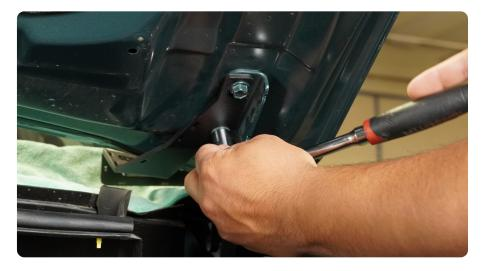
STEP 7 | Slowly and carefully close the hood and check the hood to fender gaps.
