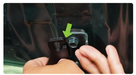
STEP 5 | Adjust the light bracket toward the front of the vehicle while ensuring the bracket does not hit the top of the hood or fender.
