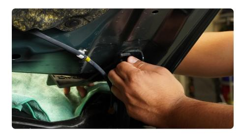
STEP 4 | Slide the brackets notched mounting points between the hood hinge and bolt head as shown.
