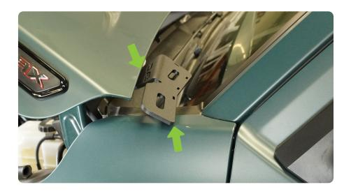
$\begin{array}{c|c} \textbf{STEP 6} & \textbf{Secure the hood hinge bolts} \\ \textbf{hand tight.} \end{array}$
