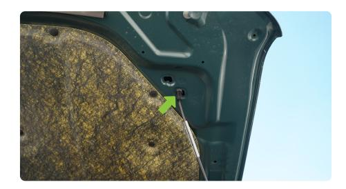
STEP 11 | Double check that all hardware is torqued to 10 ft lbs.
