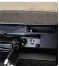
STEP 23 | If you are planning to run a winch, install the provided winch plate at this time. Using a 21mm/22mm socket and the provided M12 hardware secure the winch plate in place.
