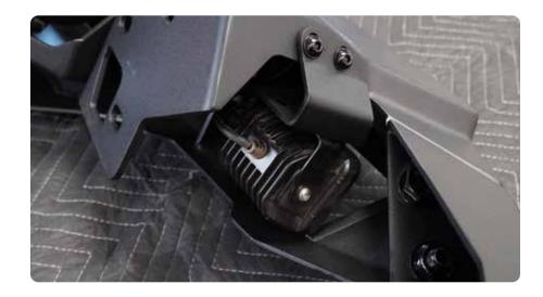
STEP 28 | With assistance mount the bumper to the vehicle. Using a 21mm and 22mm socket or wrench with the provided M14 bolts, loosely secure the bumper to the vehicles frame rails.
