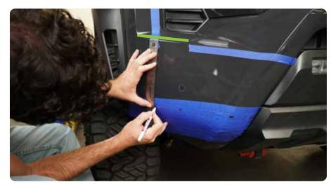
STEP 7 | Measuring from the upper corner where the bumper meets the fender, below the headlight. Make a mark at 17 7/8 inches
