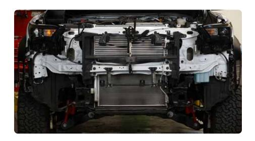
STEP 21 | with the bumper/grille assembly removed from the vehicle we can now assemble the bumper.
