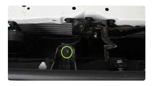
STEP 12 | Use a 10mm socket to remove the (4) bolts on each side securing the inner fender to the front bumper.
