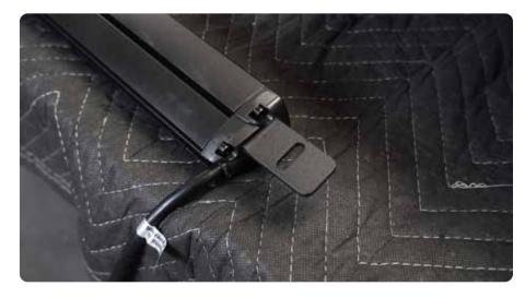
STEP 22 Using a #4 allen tool and 10mm socket or wrench, mount the light bar into the DV8 front bumper using the provide M6 hardware.
