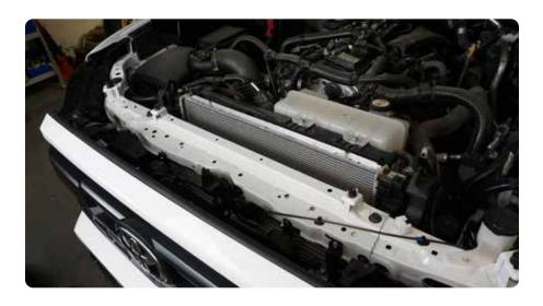
$\begin{array}{c|c} \text{STEP 10} & \text{Disconnect the 2 electrical} \\ \text{plugs connected to the grille.} \end{array}$
