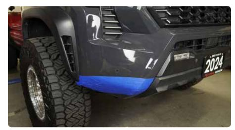
STEP 2 | Place additional pieces of tape as shown following the body lines. These pieces will help ensuring the measurement are accurate as possible.
