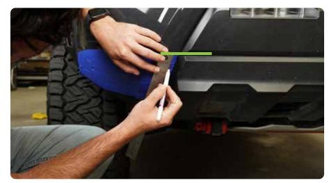
STEP 4 | Measuring from the top of the tap line down, make a mark at 67/8 inches.
