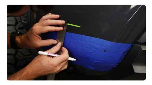
STEP 6 | Measuring from the body line down, while using the tape line to ensure you the measurement is straight with the vertical body line, make a mark at 7 3/4 inches.
