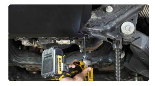
STEP 30 | Using a #5 allen tool and a 13mm socket or wrench, secure the (4) M8 bolts that secures the skid plate to the bumper.
