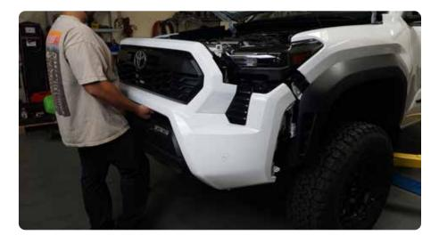
STEP 19 | Use a 17mm socket to remove the (8) bolts securing the crash bar.
