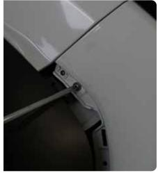
STEP 16 | Use a 10mm socket to remove the (2) bolts securing the lower bumper valance.
