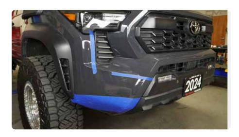
STEP 3 | Measuring from the top of the lower valance down, make a mark at 1 1/4 inches.
