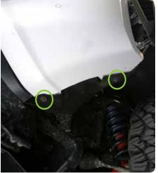
STEP 13 | Use a trim pry tool to remove the (2) push pins on each side securing the factory flare to the bumper (If equipped).
