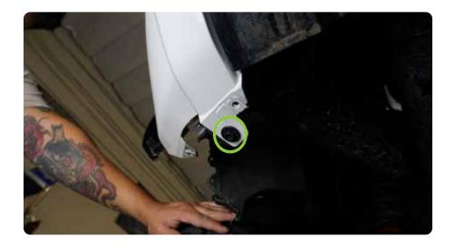
STEP 15 | Pull the front of the fender flare down to expose the Phillips head screw securing the side of the front bumper to the vehicle. Use a Phillips head screw driver to remove the screw from each side.
