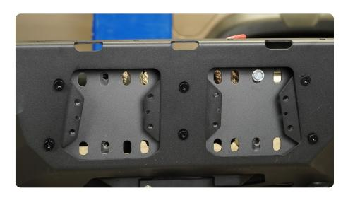
STEP 32 | Mount the cover plates to the bumper using the provided M8 counter sunk allen head hardware.
