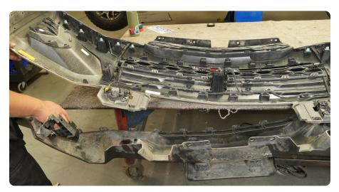
STEP 19 | This OE body line is what will be used as our "cut line" for the Spec series bumper.
