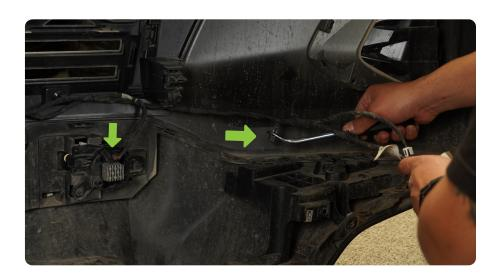
STEP 17 | Use a 7mm socket to remove the bolts on each side that hold the two portions of the bumper together as shown.
