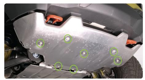
STEP 7 Using a T15 torx tool, remove the (8) bolts that secure the bottom the bumper to the vehicle.
