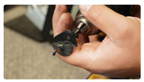
STEP 41 | Reinstall the blade mount onto the motor same as factory, and using the M5 long bolt the mount onto the motor mount.
