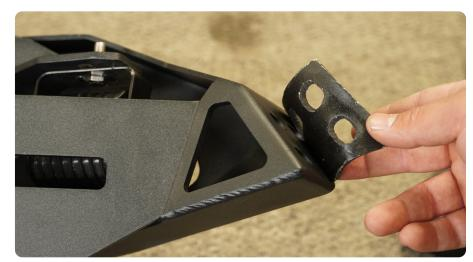
STEP 27 | Using the provided M10 hardware, loosely secure the wing to the bumper. Use (1) M10 flat washer per bolt. Use (1) M10 flat washer for each nylon lock nut.
