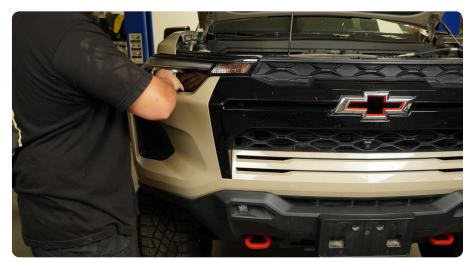
STEP 9 | With all bumper clips undone, angle the bumper/grille assembly away from the vehicle to gain access to the front camera and fog light wiring harness on the driver side front corner.
