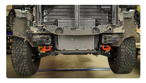
STEP 15 | Using a 18mm socket and an adjustable wrench, remove the factory recovery hooks.
