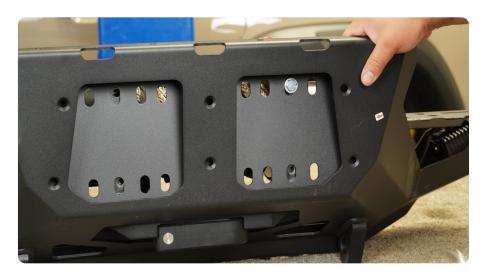
STEP 31 | Install the 3 provided cover plate mounting brackets using a #5 allen tool and the provided M8 counter sunk bolts.
