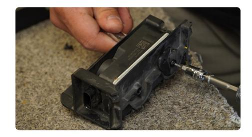
STEP 44 | Slide the air dam motor into skid plate bracket, secure the air dam motor using the provided M6 hardware.
