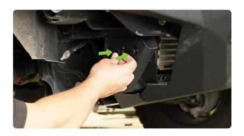
STEP 48 | Using a 18mm and 19mm socket or wrench, secure the M12 bolts.
