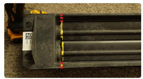
STEP 37 | Remove the housing from the motor/shutter blades.
