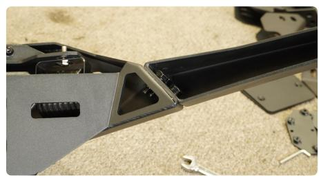
STEP 29 | If you are planning to run a winch, install your chosen fair-lead at this time using the hardware this is included with the fair-lead kit.
