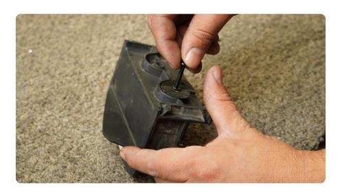
STEP 42 | With the bolt inserted, press on the backside to score the housing and using the 3/16": drill bit, carefully drill though to allow the bolt to be through bolted.
