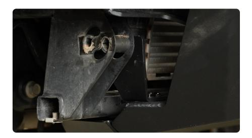
$\begin{array}{c|c} \text{STEP 47} & \text{Place the provide cap over} \\ \text{the recovery hooks brace}. \end{array}$
