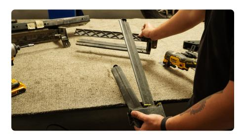
STEP 38 | Remove the shutters blades from the air dam motor.
