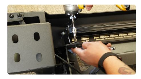
STEP 26 | Place the provided foam pieces on to bumpers wing mounting points as shown. Ensure the shape of the foam is matched to the shape of the mounting point.
