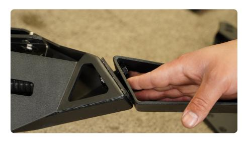
STEP 28 | Adjust the wing so that the wing and bumper are aligned at the front. Using a 16 and 17mm socket or wrench secure the wing in place.
